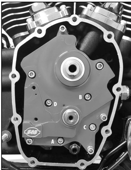
Picture 3b: Oil Pump Screws-Torque According to Step 34
