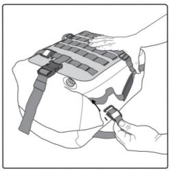
6. Once all straps are secured to your vehicle, pass the cam hook through the loops on the side of the bag to help minimize your bag movement.
