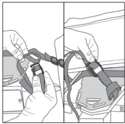
5. Loop one of the four Rigg Straps® around a rack or a secure location on your vehicle. Pass the cam hook through the loop on the long strap end and pull to secure. Repeat with other 3
