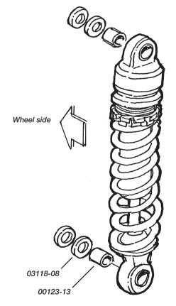
Normaly the shock absorber is mounted with the cylinder head upwards. Check that there is enough clearence to other details both in loaded and unloaded position.
