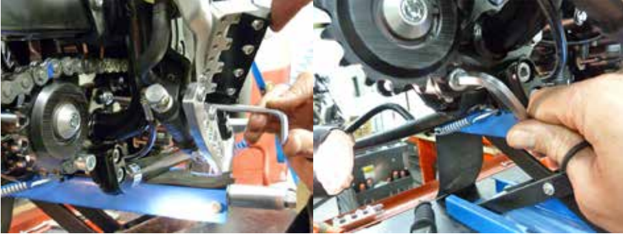
Secure the chain tensioner.
