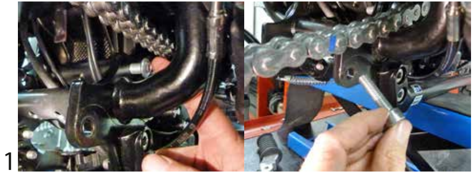
1 Insert bottomhead bolts m10x45 in the holes of the frame as in the photo
