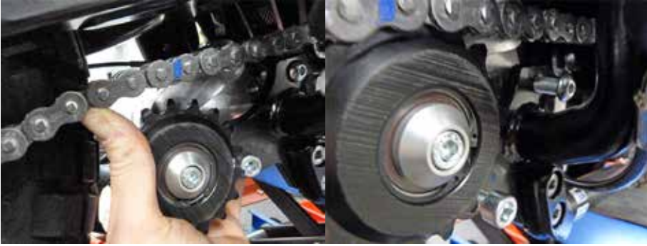
Position chain tensioner by aligning the threaded holes.
