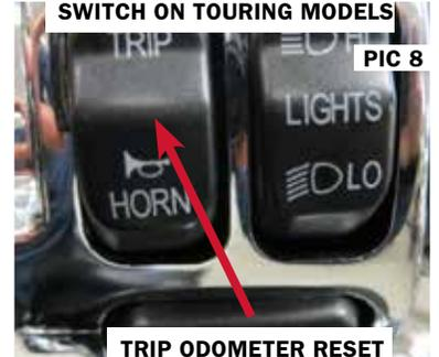
**TRIP ODOMETER RESET SWITCH ON SOFTTAILS, SPORTSTER AND DYNA**
