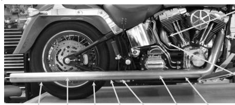
NOTE: Arrows point to HS-28 the position of the hex CLAMP head of the clamps.
