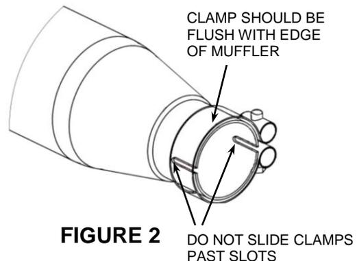
POSITION OF MUFFLERS AND MOUNTING BRACKETS SHOWN ABOVE MAY VARY FROM ACTUAL APPLICATION
