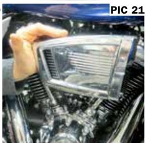
**STEP 21** Refer to PIC 22. Locate the two (2) socket head cap screws that were removed in Step 16. Insert the screws into the outside edge holes of the cone. As you tighten the screws the cover should pull forward, closing the gap between the cone and cover. Fully tighten all four (4) screws in the cone.
