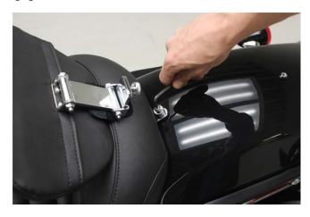
3. Align the rear bracket with the rear fender nut and secure with the stock screw.
