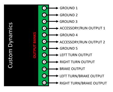
Use a small straight slot screw driver in the output port selected and turn the screw counter clockwise until the wire slot is open.
