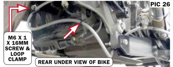
**STEP 33** Refer to PIC 26. Secure any slack in the brake line to the bike. Be sure to fasten the brake line where it won't pinch, pull, rub, or be damaged.
