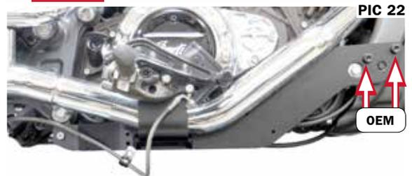
**STEP 29** Locate provided M8 x 1.25 x 50mm screw and M8 Lock Nut.
