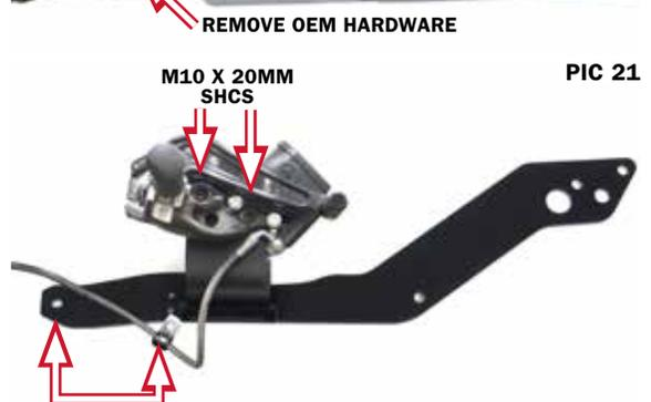
**STEP 27** Align the Right Bracket assembly with the bike and determine how and where the brake line will be re-routed.
