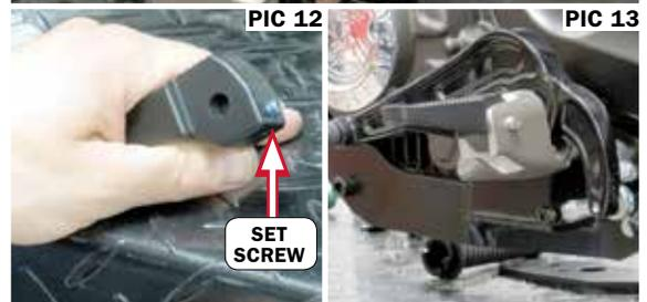
**STEP 15** Refer to PIC 12 and 13. Locate one (1) provided footpeg. Adjust the set screw in the back of the peg to adjust the sitting position of the peg. When it is set, align and place the footpeg into the mount, and secure it in place with the pivot pin and retaining ring that was removed in Step 14.
