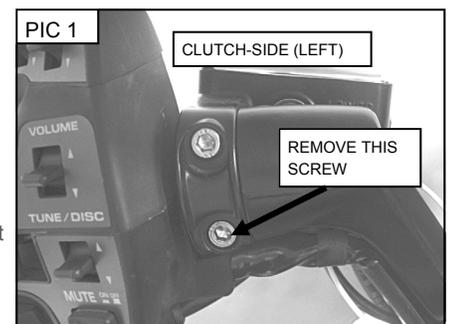
**STEP 4** Compare the threads of the included screws with the threads of the existing screws to determine the correct screws.
