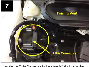
Locate the 2 pin Connector to the lower left (looking at the fairing) of the vent on the motorcycle. See photo item circled for connector location.
