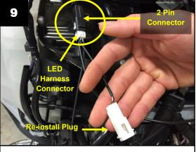
Plug the Vent LED Harness Connector into the Fairing 2 pin connector, ensure that it Snaps in. Make sure to reinstall the plug removed in step 3 into the LED harness pass-through connector.
