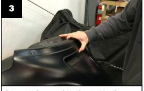
Remove the front outer fairing from the bike, if unsure of this process, please refer to manufacturer service manual for details.
