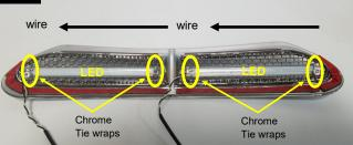
Place the vent trim upside down on a padded work surface as shown. Make sure surface is protected so as not to scratch vent. Unwrap the harness assembly and stretch out end to end. Notice that one LED wire is longer than the other, this LED will install first on the right side. Make sure the wires are facing the direction in the photo.
