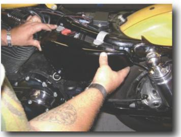
14. Reinstall the bike's side cover and the rear fuel tank mounting bolt. Torque the rear mounting bolt and the front bolt /nut previously loosened to 15-20 ft-lbs (20.4-27.1 Nm) Reconnect the battery, torque battery terminals to 60-96 in-lbs. (6.8-10.9 Nm).
