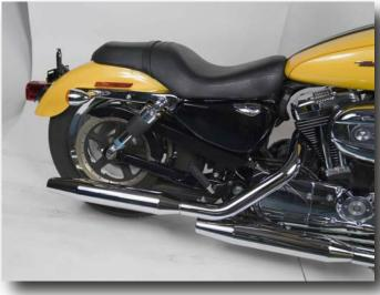
16. Make sure that there is adequate tire to rear fender clearance. Check both the center of the tire and the sides with the system in the lowered position, with zero air pressure.
