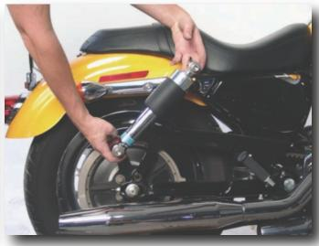
2. Install the new air suspension shocks one at a time. Start with the lower bolt holes first. Then raise or lower the bike to line up the upper bolt holes.
