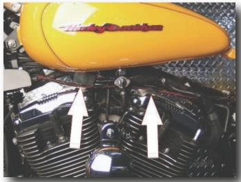
7. After connecting the 4mm air tubing to the compressor, route it beneath the left side of the fuel tank and along the frame toward the rear of the bike. Step #8 will cover connection to the distribution block using one of the 4mm VOSS®
