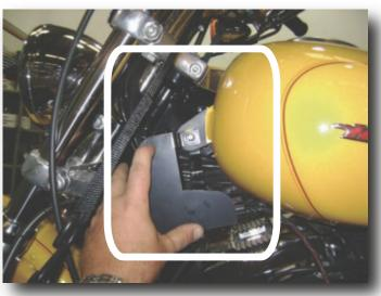
4. Place the compressor assembly over the front mounting bolt. Replace the mounting nut but leave loose for now.
