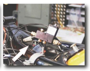
8. A preferred location for the solenoid vent valve/distribution block is under the seat.
