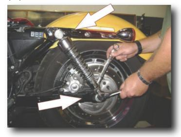
1. Loosen and remove the upper and lower shock bolts.
