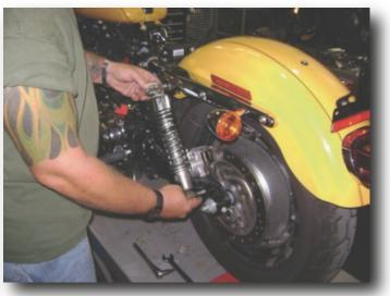
2. Carefully remove factory shock absorbers from the rear suspension.
