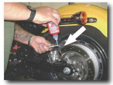
1. Remove the new  $\frac{1}{2}$  X 3" shock bolts and washers from the kit. Apply 2-3 drops of Loctite® 243 (blue) to the threads of each bolt. Torque all shock bolts to 45-50 ft lbs (61.1-67.9 Nm).
