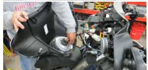
*Note: Be careful to not bump the fairing against the signal lights or other installed lights connected to the front fork. A sock or other fabric can be used to protect the side lights during fairing removal.*
