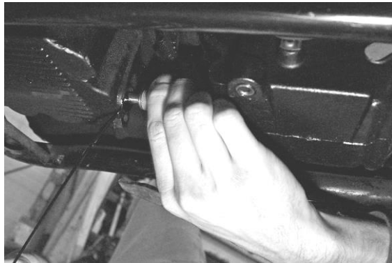
Thread sender into oil pan
