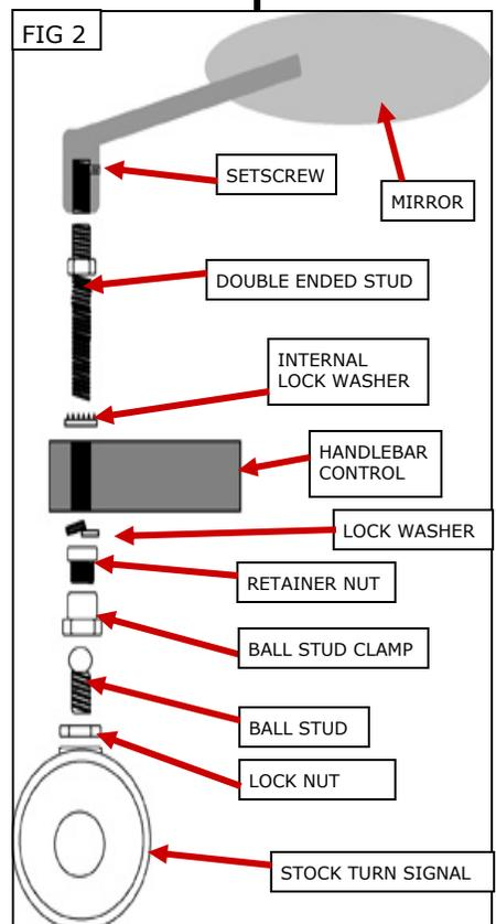
**STEP 12** Screw a double ended stud into the new mirror stem; tighten and then tighten the set screw.
