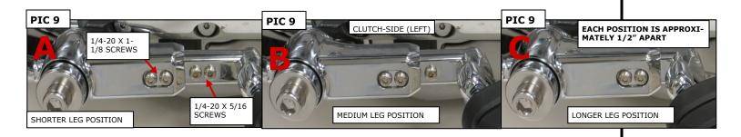
**STEP 11** On the clutch-side of the bike, attach the Extension Arm to the Rotating Arm with two of the included 1/4"-20 X 1-1/8" Button Socket Head Screws. Thread the screws through the Extension Arm and secure them on the back side with two of the included Nylock Nuts. Fill any exposed threaded holes with the included 1/4"-20 X 5/16" Button Socket Head Screws. **PIC 9 A**
