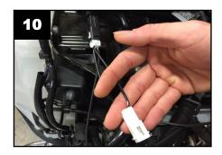
Having an extra set of hands is helpful for the next steps. The outer fairing will have to rest near the Inner fairing in order to make the wire connections. One person should hold the fairing in place, while the other performs the connections.
