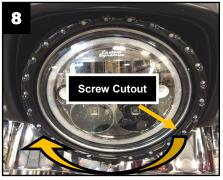
Mount the trim ring to the headlight assembly. Align the screw cutout to the right as shown in figure 8, then push and turn the trim ring clockwise until the screw hole is aligned with the mounting arm at the bottom and the top attachment W clip (figure E page 2) seats in the retainer of the headlight bracket. You may need a flashlight to see inside to confirm alignment for the mounting screw.
