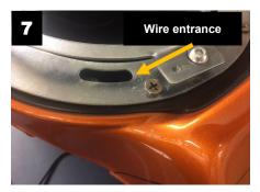
Feed the head light trim ring wires through the small opening on the headlamp mounting frame shown in figure 7.
