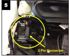
Locate the 2 pin connector to the lower left (looking at the fairing) of the vent on the motorcycle. See photo item circled for connector location.
