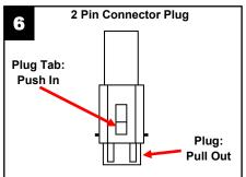
Remove the connector plug from the connector on the motorcycle by pushing the center tab in and pulling the plug out. Save the plug for reinstallation in step 7.
