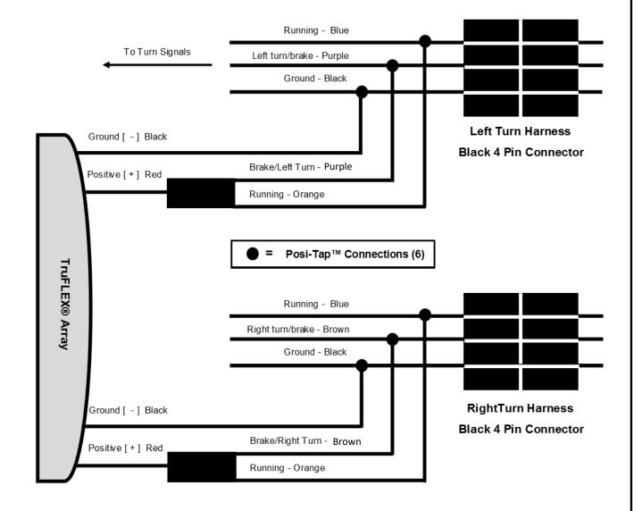
This product is designed and intended for use as auxiliary lighting on motorcycles only. This product is NOT intended to replace any original equipment lighting installed on the motorcycle and should not be used for that purpose. This product must be wired such that it does not interfere with any original equipment lighting.
