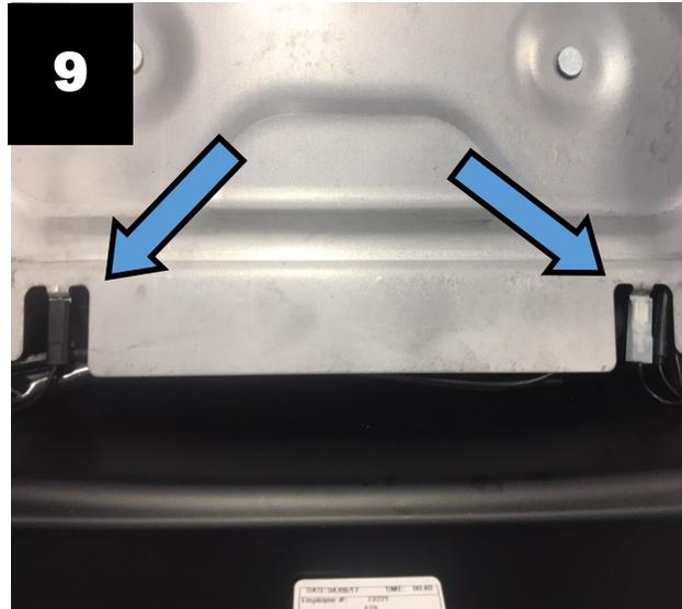
9. Remove ground wires from mounting plate .
