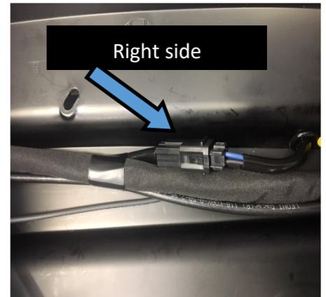
10. Disconnect 2 pin factory wire harness to the Tour Pak® lights.
