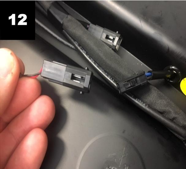
12. Connect the **longest** 2 wire harness with the 2 pin female plug of the MAGIC-TPC-LED to the LEFT side marker light 2 pin male plug.
