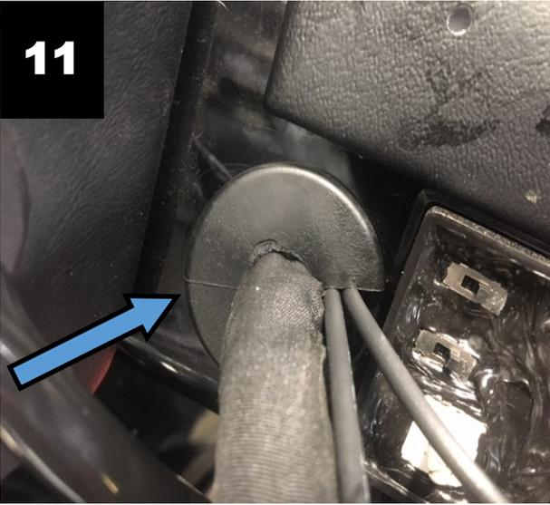
11. Remove grommet from right side of Tour Pak®. Save to re-install at a later step.
