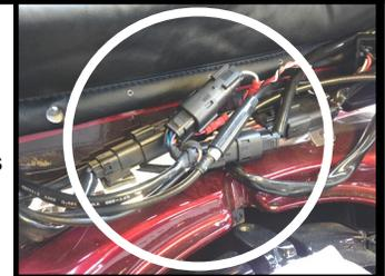
**Note:** Some 2016 models and all 2017-2020 models will not have a (y) configuration harness, there is only one 6 pin harness connector in this location, which is the correct plug for the Magic Strobes™ unit.
