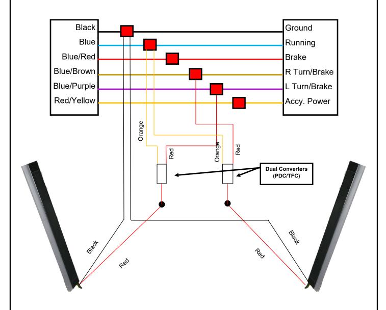
Note: This diagram demonstrates run/brake/turn with (2) TFC dual converters (each sold separately).
