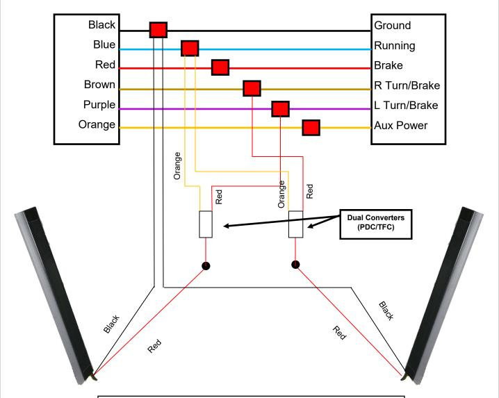
This diagram demonstrates run/brake/turn with the MPR-BCM adapter and (2) TFC dual converters (each sold separately). Other Functions available:
