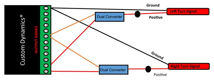
**Dual Converter** Orange—Running Light Red—Brake/Turn
