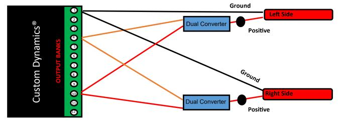
**Dual Converter** Orange—Running Light Red—Brake
