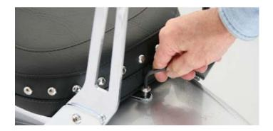
6. Place the white nylon washer under the passenger seat's rear bracket and secure with the stock 6mm bolt. Tighten securely using a 5mm Allen wrench.
