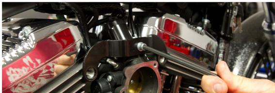
3. Disassemble Comp-V to backing plate.
