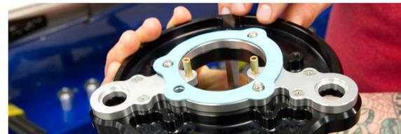
5. Loosely install Comp-V backing plate. Some resistance is normal with the thread lock compound on bolts.
