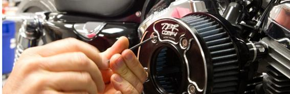
11. Apply anti-seize to threads of plug cap or v-stack and install hand tight.
