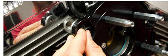
7. Install o-ring onto end of each oil channel spacer.
