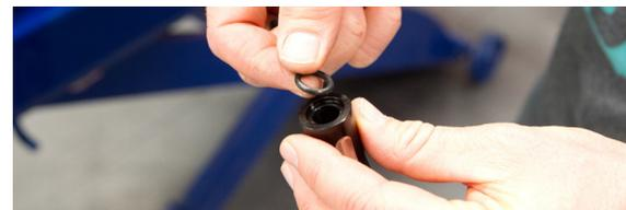
8. Apply loc-tite to banjo bolt threads. Put banjo bolts through backing plate and spacers. When installing backing plate to throttle body be sure to tighten socket head screws and banjo bolts evenly 1/4 turn at a time to ensure no binding. (Socket head screws are self locking and some slight resistance is normal when tightening.)
