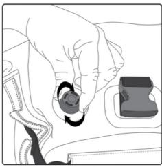
2. Open the air valve a 1/4 turn to allow bag to compress. Be sure to close when done and not over tighten.
