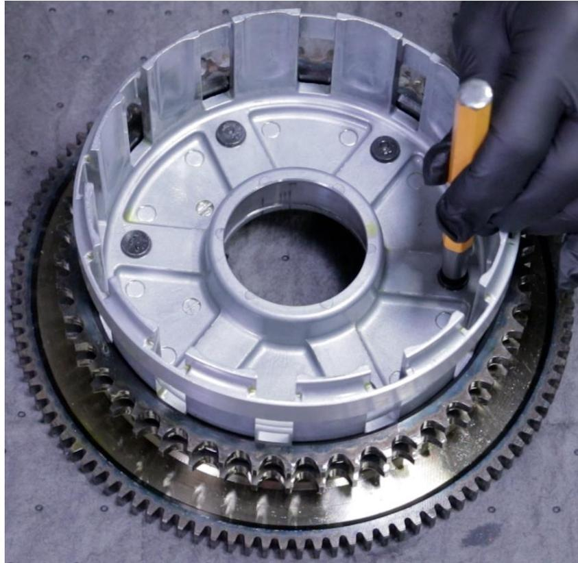
**Note:** Center punching and drilling on the ring gear side can lead to damage of the ring gear and potential failure of the new clutch basket. By drilling on the inside of the basket it is easier to maintain the integrity of the ring gear.
