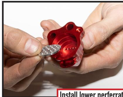
Install lower perforated disc (smaller) into breather body. Make sure disc is flat and fully in place inside housing
