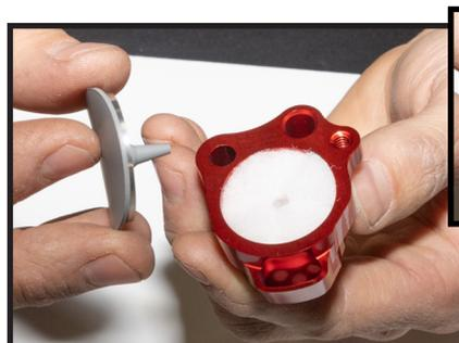
Install umbrella valve and disc on top of filter element.
