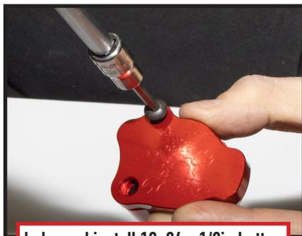
Lube and install 10-24 x 1/2in button head to seat aluminum cover.
