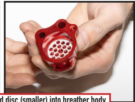
2. Assemble cylinder head breathers: Lower disc, Filter element, Upper disc, Umbrella valve, Top cover and Hardware.
