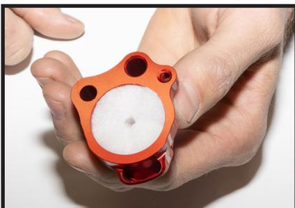
Install filter element into breather body. Fully tuck in edges of filter elements so there is no excess material showing.
