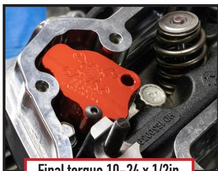
Final torque 10-24 x 1/2in button head to 22-24 in/lbs.
