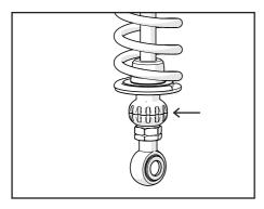
Rebound damping:-Bottom Adjuster Wheel:- 32 clicks adjustment range. All settings should be made from the fully closed (Clockwise Position).
