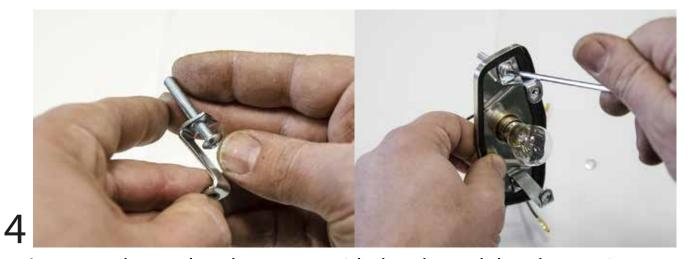
Insert m5 bottonhead screw provided and attach bracket again.
