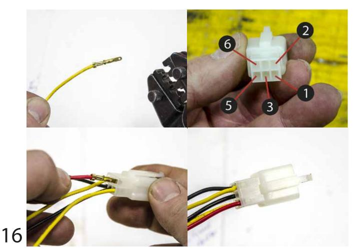
Attach two connectors on indicators wire remaining. To build the plug following the diagram, see on page 9.
