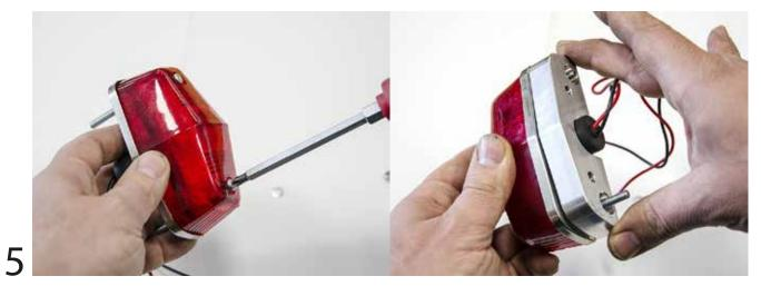
Reassemble tail light and Insert provided base as photos.
