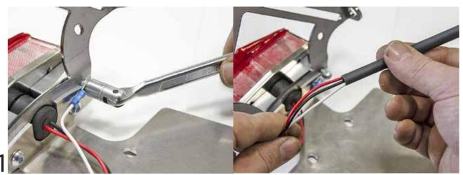
Tighten nut and insert wiring into the sheath as photo.
