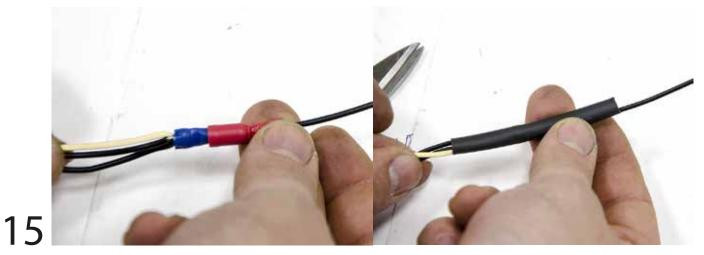
Connect cable as photos and apply the sheath.
