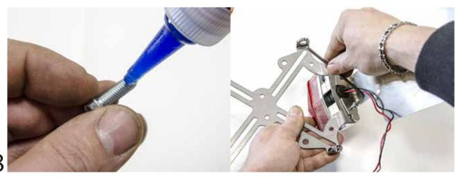
Apply thread lock to M6x16 bottonhead bolt and fix support plate on undertail as photo.
