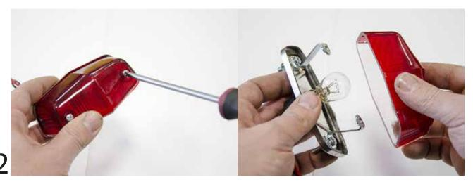
Disassemble new tail light as photos.
