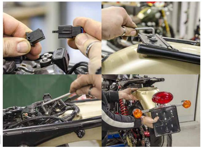
Before installing you must first disconnect negative lead from the battery. Disconnect rear lights plug and remove fender.
