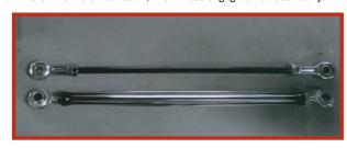
4. Install the RSD shift rod using the factory hardware. Use blue threadlocker on the bolts and torque to 15 ft-lbs. Once both ends are installed tighten the jam nut using a 1/2" wrench.
