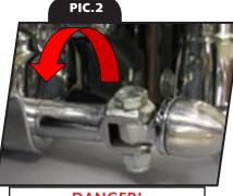
DANGER! THIS TYPE OF FOOTPEG MOUNT WILL "TWIST" AND LOOSEN THE FASTENER SECURING IT TO THE MOTORCYCLE.
