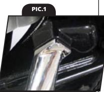
GOOD! THIS TYPE OF FOOTPEG MOUNT CANNOT "TWIST" AND LOOSEN THE FASTENER SECURING IT TO THE MOTORCYCLE.
