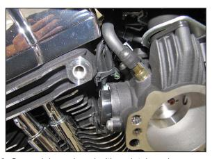
6. On models equipped with an intake valve solenoid connector on the back of the stock air filter back plate; unhook the connector from back plate and use the provided tie wrap to secure it behind the throttle body.
