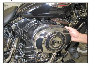
2. Remove air filter cover mounting bolt and cover from the vehicle as shown.
