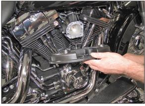
5. Remove the stock air filter base and gasket from the engine as shown.
