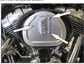
3. Remove the three bolts which secure the stock air filter element. Then remove the stock air filter element and stock crank case breather hoses as shown.
