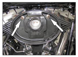
4. Remove the stock breather bolts which secure the stock air filter base shown.
