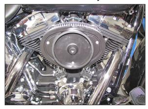
11. Install the  $K\&N^{\otimes}$  air filter and secure with the three bolts provided.
