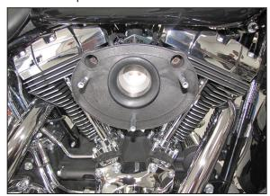
10. Install the back plate and secure with the stock breather bolts. Tighten the three bolts that secure the back plate to the throttle body. Then tighten the two breather bolts fully.
