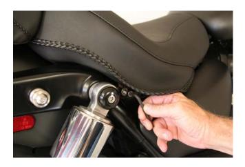
5. Align the solo's side brackets with the mounts on either side and install the stock 6mm bolts. Tighten both finger-tight, then tighten securely with a 5mm Allen wrench.
